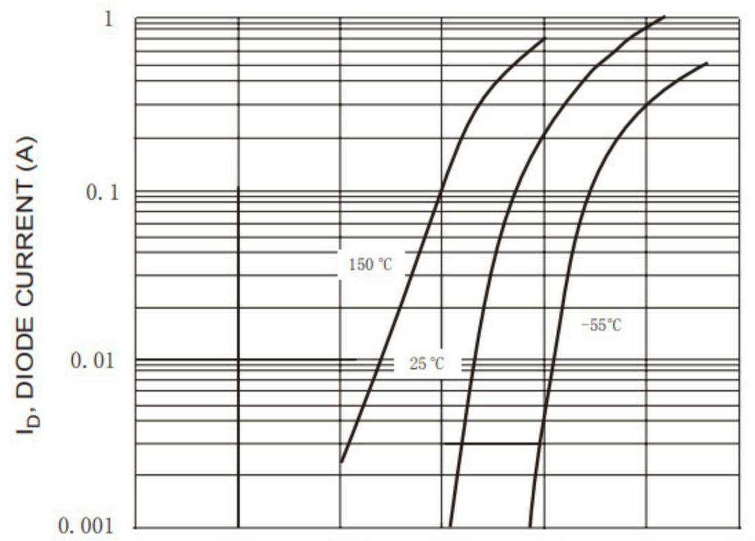
Fig. 9 Body Diode Current vs. Body Diode Voltage
