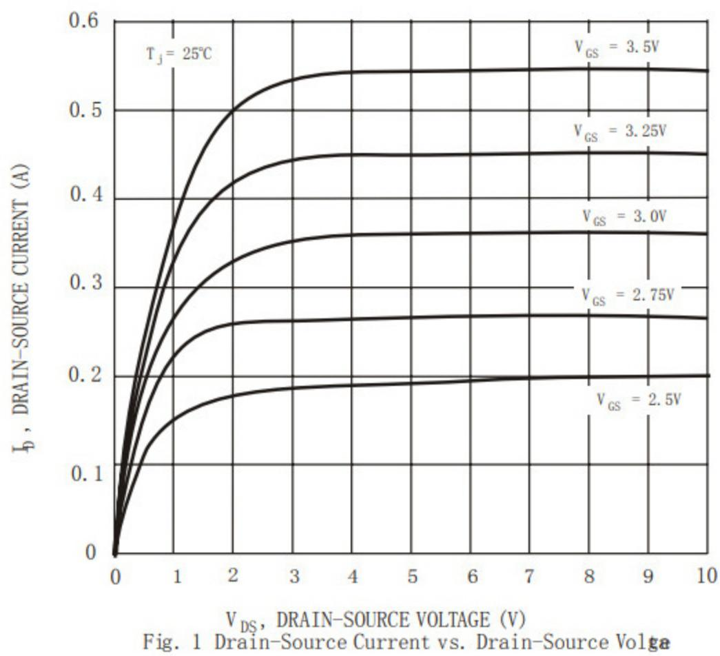
Fig. 1 Drain-Source Current vs. Drain-Source Voltage
