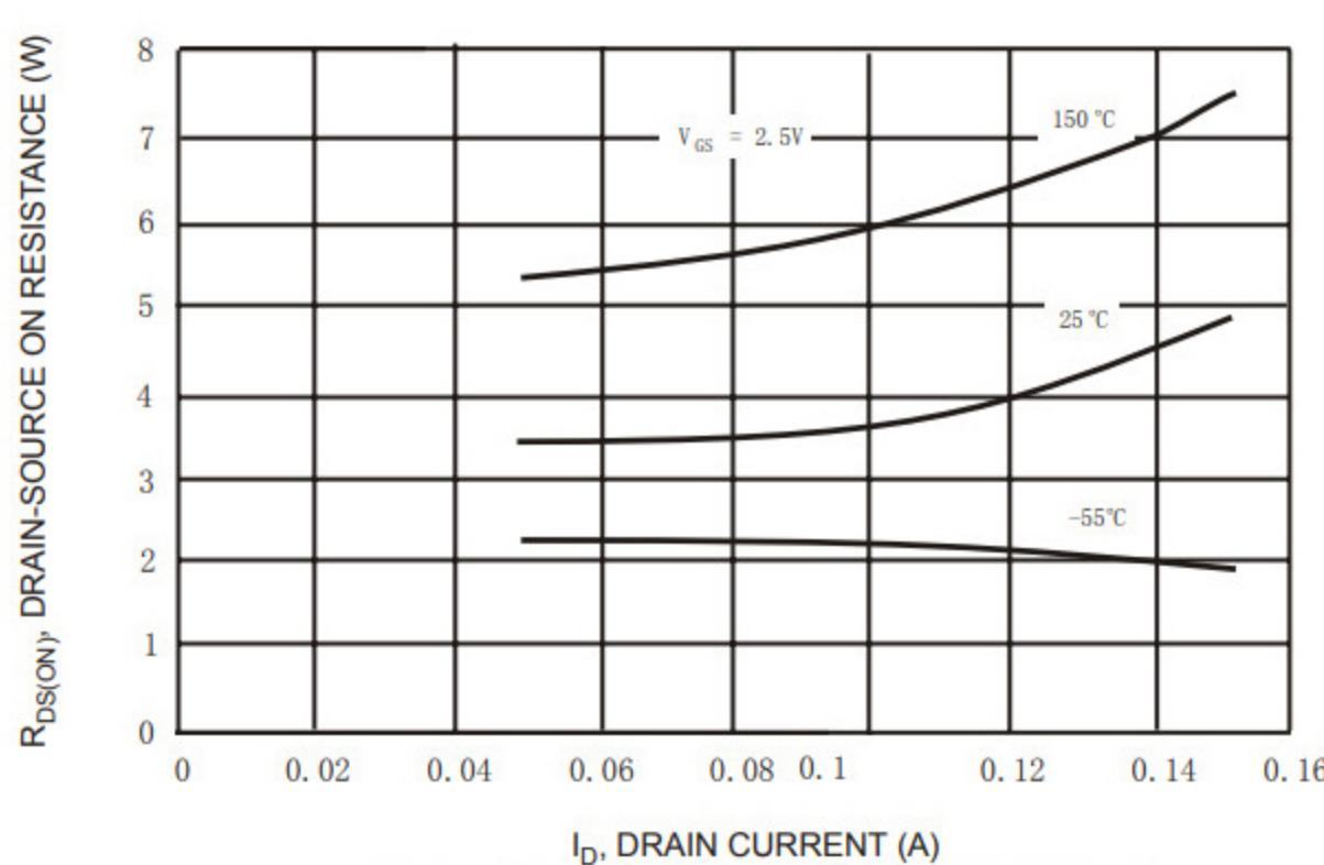
Fig. 5 Drain-Source On Resistance vs. Drain Current
