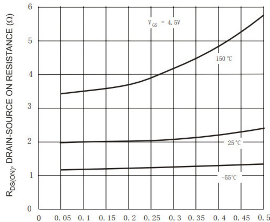
Fig. 7 Drain-Source On Resistance vs. Drain Current
