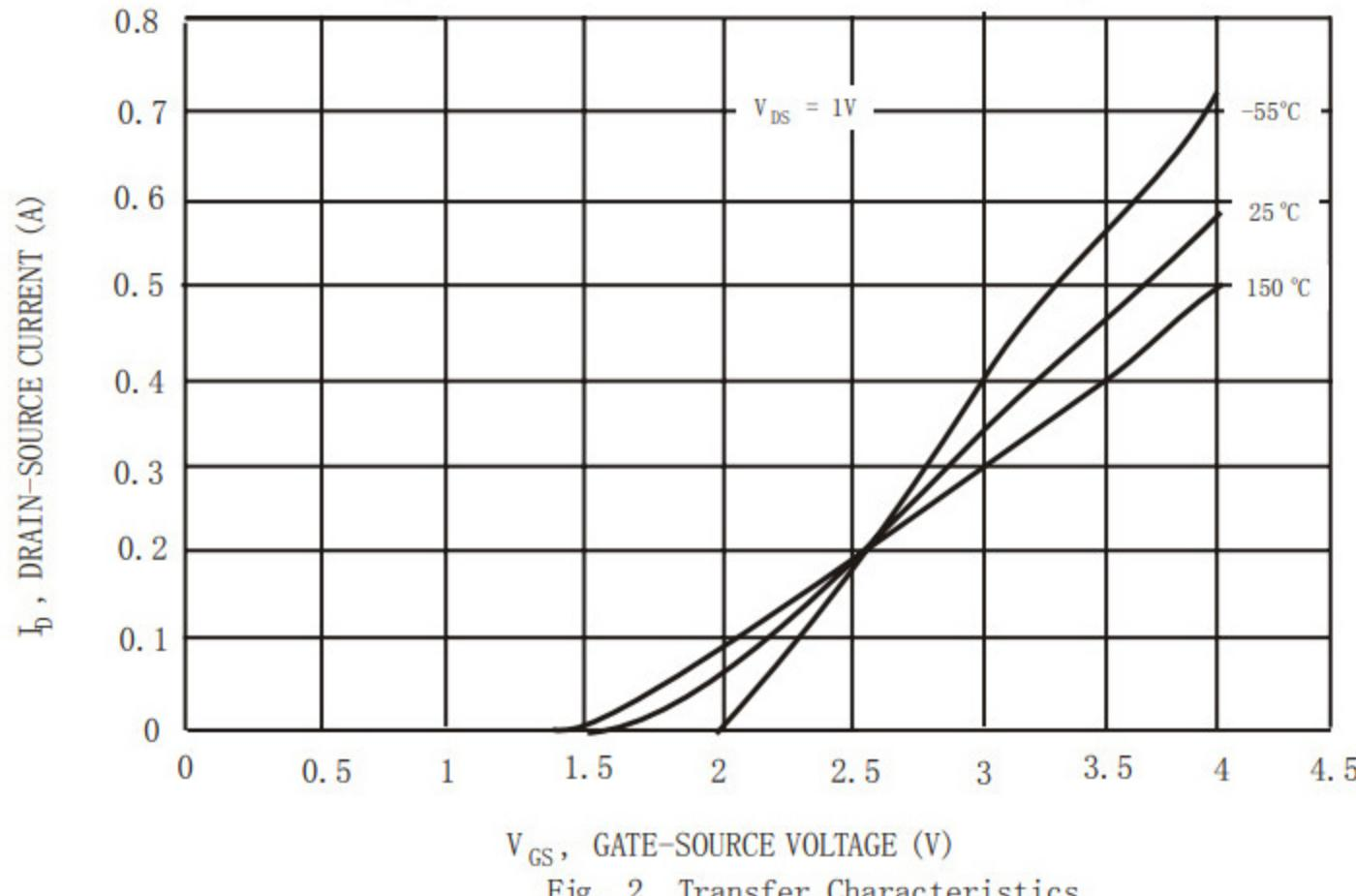
Fig. 2 Transfer Characteristics
