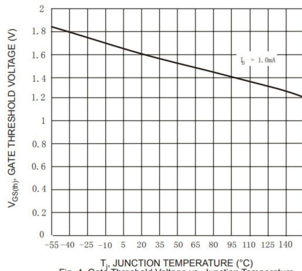
Fig. 4 Gate Threshold Voltage vs. Junction Temperature
