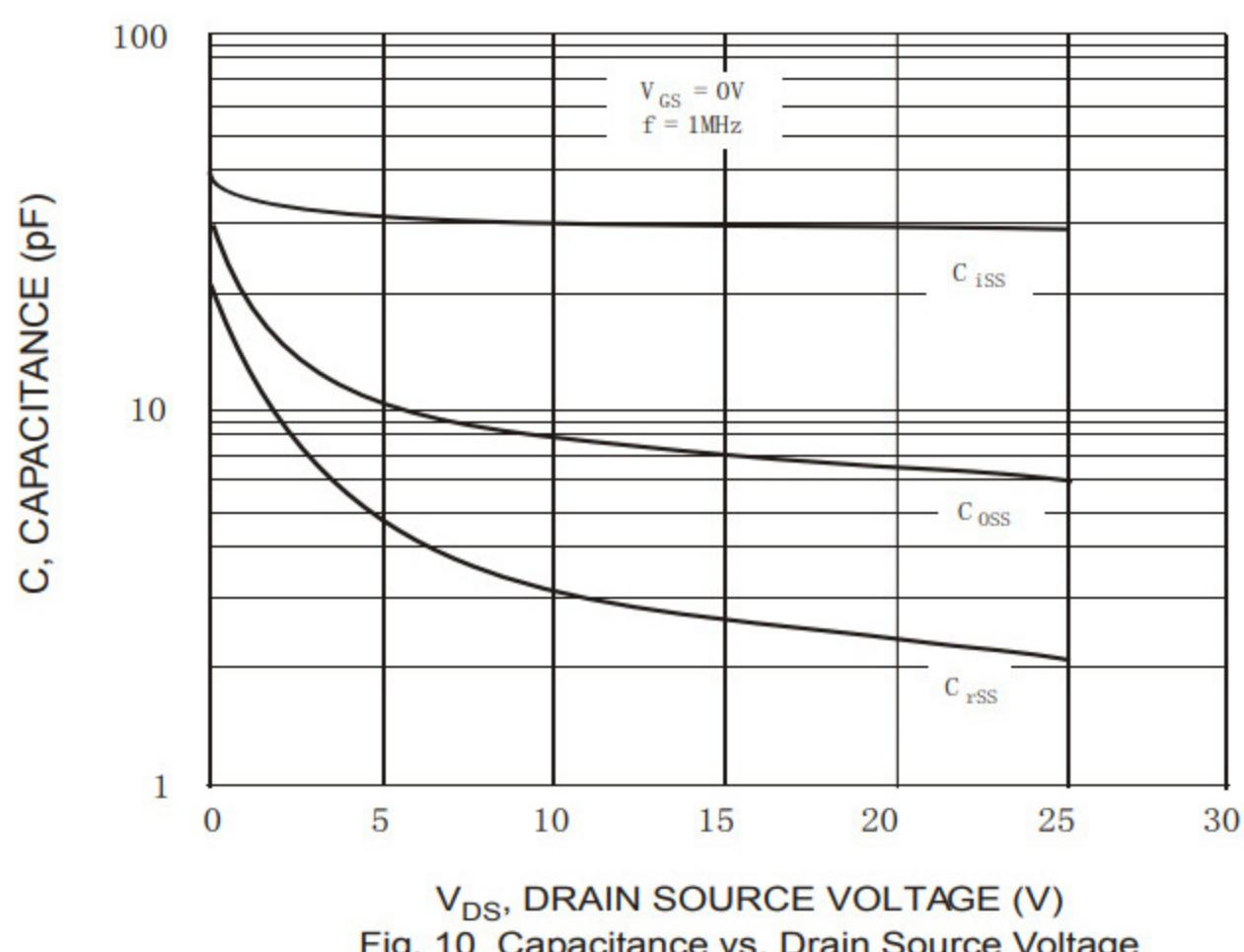
Fig. 10 Capacitance vs. Drain Source Voltage
