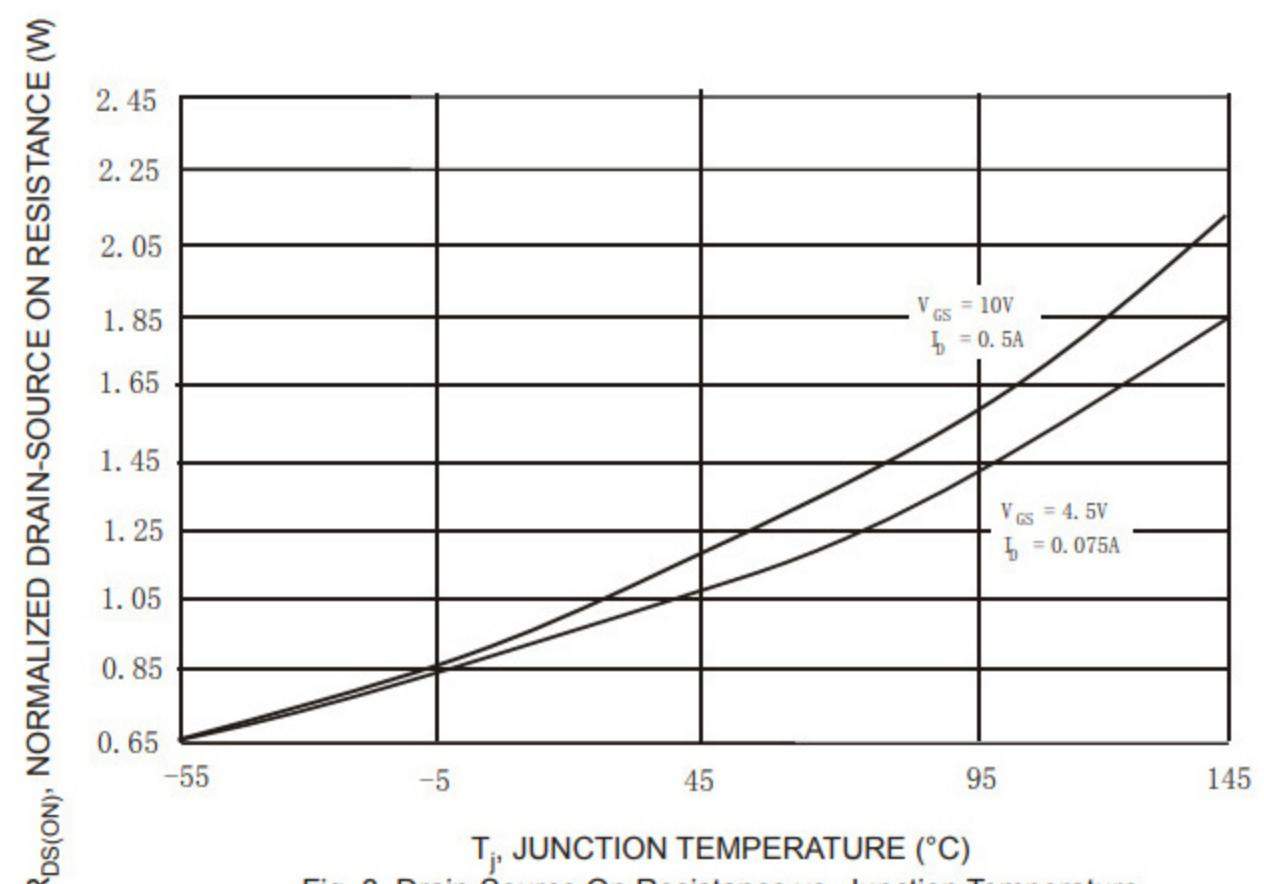
Fig. 3 Drain-Source On Resistance vs. Junction Temperature
