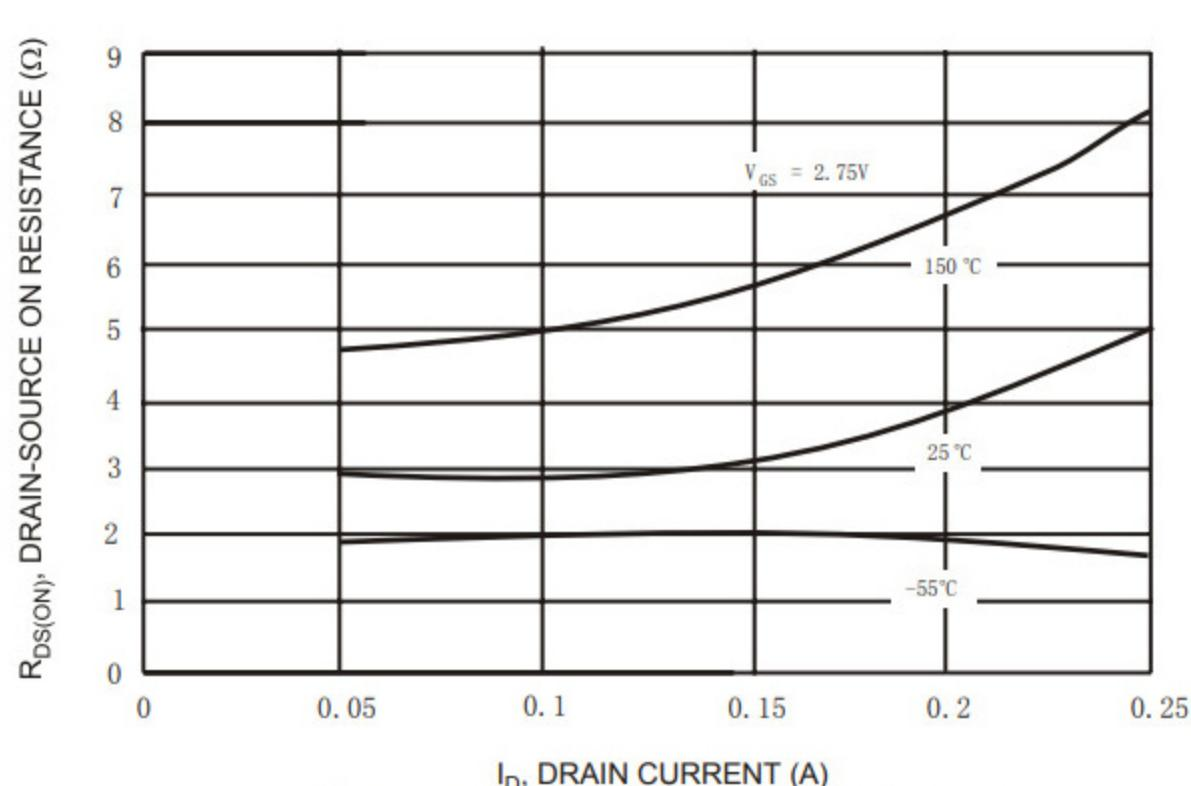
Fig. 6 Drain-Source On Resistance vs. Drain Current
